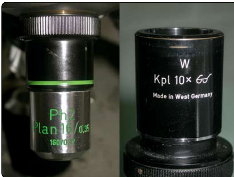
(L) Example of an objective lens, with text describing the lenses functions: Ph2 = phase contrast lens (which I'll describe in an upcoming installment), and phase ring size, Plan = plan achromatic lens, 16 = 16X magnification, 0.35 = 0.35 NA, 160 = for 160 mm microscope tube, 0.17 = use with 0.17 mm slide cover. (R) Example of an ocular lens, with text meaning: W = widefield, Kpl = (Zeiss-specific code) use with plan objective, 10x = magnification, (glasses) = high point focus.. Photo by Peter Werner
