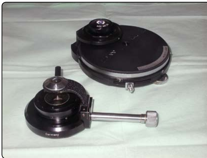
My condenser collection: (front) What I use mostly—typical Zeiss “flip-top” style Abbe condenser, with a 0.9 NA “dry” top lens, and lower lens with even lower NA for illumination of low-magnification objectives; (back) for really good images—turret style phase contrast/darkfield/brightfield condenser, with 1.4 NA dedicated oil-immersion achromat/aplanat top lens (not necessarily easy to set up and clean, but the image quality—WOW!). Photo by Peter Werner
